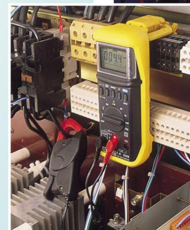
◀ Measurement of an AC current in complete simplicity with the miniclamp MN 89 combined with the C.A 5230G, suspended from its folding clip.
