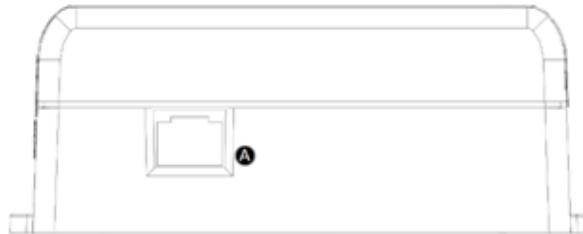
Figure 13 - RF542 RJ45 Network Port
