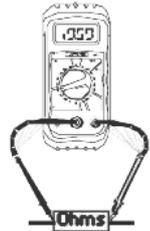
4. Read the resistance in the display and then set the function switch to the lowest W position that is greater than the actual or any anticipated resistance. The display will indicate the proper decimal point and value.
