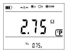
The  $\rightarrow 0 \leftarrow$  symbol blinks during the compensation. When it is done, the display unit indicates **00.00** $\Omega$ .
