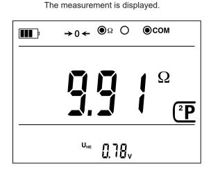
The instrument displays the measured value minus the compensation.
