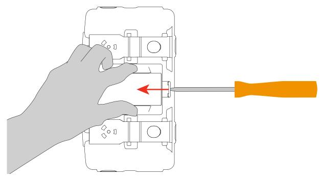
Remove the battery compartment cover, then raise the rubber plug.
