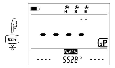
Move the S rod towards the H rod by 10% of d and make another measurement. Press the 72% key to store it. Then move the S rod again by 10% of d, but towards the earth electrode. Make another measurement and press the 52% key to store it.
