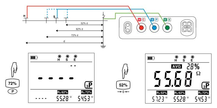
The instrument immediately calculates the mean of the 3 measurements and the percent difference between the lowest value and the highest value. For the measurement to be valid, the difference must not exceed 5%.
