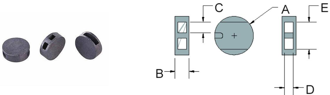
The Round Lead Seal is designed with two parallel holes and a knot chamber. During fitting the wire or string is threaded through the two smaller holes and crossed inside the knot chamber before closing with the sealing tool to prevent slippage.
