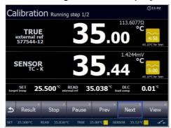
When the temperature has reached the stable criteria, the calibration data will be stored and the temperature goes towards the next set temperature.
