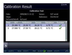
The calibration results can be uploaded with the "JOFRACAL" PC program. This enables you to print out the results on a certificate.
