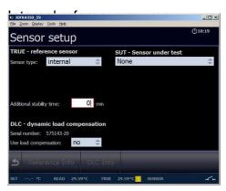
The internal reference sensor will be displayed as the TRUE value on the main screen.
