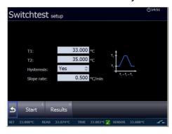
If no change in the switch position is registered during the test a red cross will be displayed in the Result list instead of a green check  $\checkmark$ .
