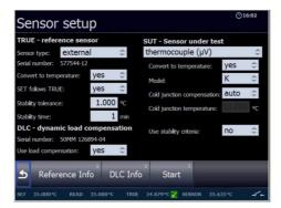
The Sensor setup menu is displayed. In this menu you have the opportunity to check and if necessary change the settings as described in section 5.7 – Sensor Setup menu.
