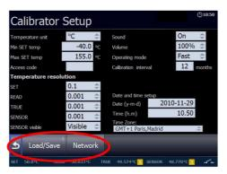
1. By pressing the ARROW UP key ▲ focus will move from the horizontal menu to the parameter field area.
