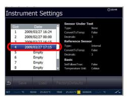
**4.** When the desired dataset in the list is highlighted press **O** or **\( \ldots**\).
