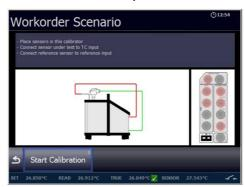
A workorder Scenario is displayed, giving a graphical display of the setup and sensor connections.
