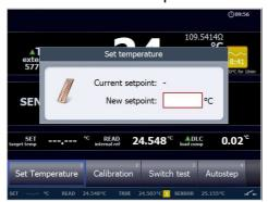
2. Use the NUMERIC keys to enter a new value, or ● or ← to accept the value. When pressing the ACTION key or the ENTER key the calibrator returns to the main menu screen.
