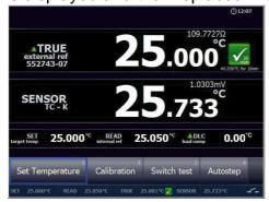
The functions in the horizontal menu are available using the soft keys or the arrow keys on the keyboard (see description in section 4.1).
