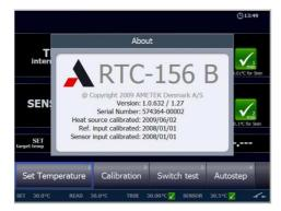
This informs you about the calibrator type, the software version installed, the serial number and the date when it was last calibrated.
