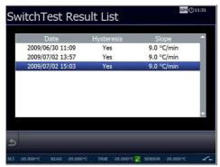
6. Scroll through the list using the ARROW UP key ▲ and the ARROW DOWN key ▼ and just press or ← to display the result of the highlighted dataset.
