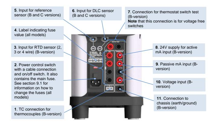
One of the inputs either pos. 1, 3, 9 or 10 can be selected displaying the "SENSOR" temperature in the Setup and pos. 5 can be displayed as "TRUE" temperature.
