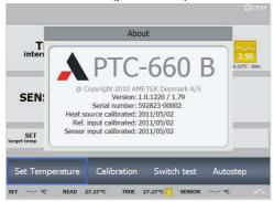
This informs you about the calibrator type, the software version installed, the serial number, the date when it was last calibrated, the build date and the build description.
