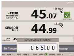
2. Use the ARROW keys to enter a new value, and to accept the value and return to the main menu screen. If pressing the BACK key the calibrator returns to the main menu screen without accepting the new value.
