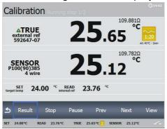
When the temperature has reached the stable criteria, the calibration data will be stored and the temperature goes towards the next set temperature.
