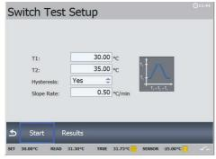
If no change in the switch position is registered during the test a red cross will be displayed in the Result list instead of a green check  $\checkmark$ .
