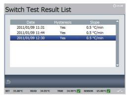
6. Scroll through the list using the ARROW UP key ▲ and the ARROW DOWN key ▼ and just press to display the result of the highlighted dataset.
