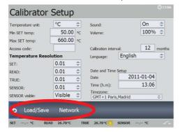
**1.** By pressing the ARROW UP key focus will move from the horizontal menu to the parameter field area.
