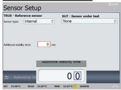
The internal reference sensor will be displayed as the TRUE value on the main screen.
