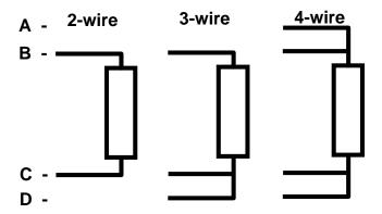
See section 10.0; Technical specifications for supported types of RTDs. The calibrator accepts 2-, 3-, and 4-wire inputs, with the 4-wire input being the most accurate.
