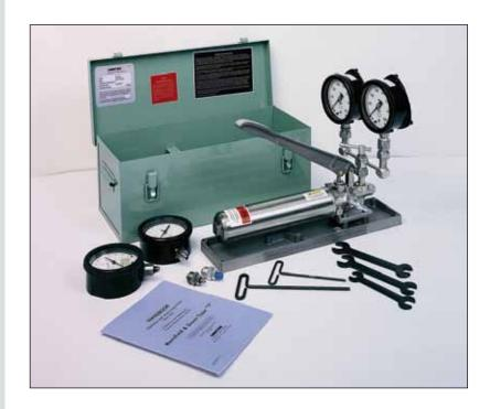
The AMETEK Comparators are ideal secondary standards for pressure measurement. The comparator test set consists of a hydraulic hand pump on a pan as the pressure source, a test manifold and a set of four 4.5 inch test gauges. Gauge PSIG spand vary with model.
