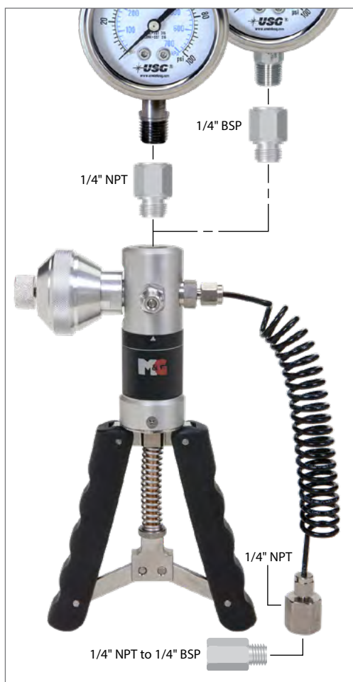
Standard fitting connection.
