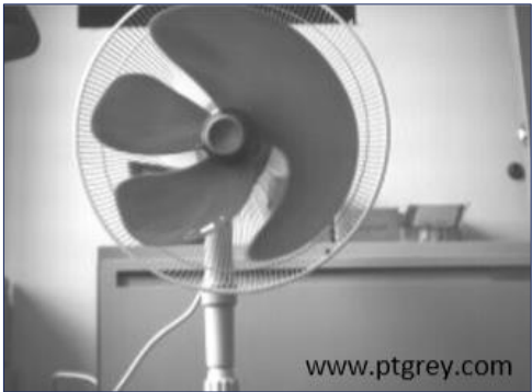
Image taken with a rolling shutter, causing the fast-moving blades of the fan to look distorted.
