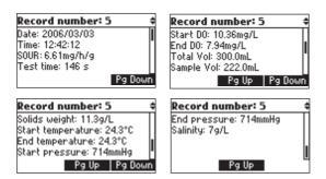
Note: In case that the SOUR value was corrected to 20 °C the message "(@20 °C)" will be displayed before the SOUR value.
