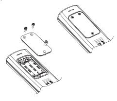
Replace the three 1.5V AAA alkaline batteries located in the battery compartment, observing the indicated polarity.
