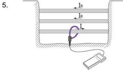
5. Place the flexcoupler around the cable that is to be identified or the phase in such a way that the arrow on the flexcoupler points towards the far end.
