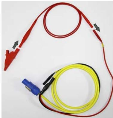
1. Remove the connection clip from the red connection cable.
