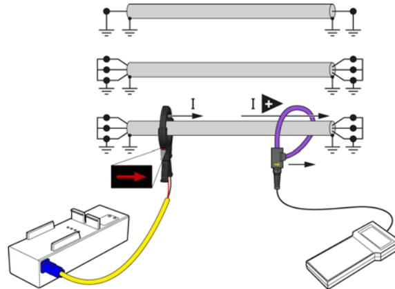
1. Place the clip-on current transformer in such a way that the arrow on the current transformer points in the direction of the far end.
