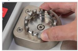
▲ The standard adjustable wire terminal fixture accommodates wire diameter sizes up to AWG 3 (0.25 in [6.3 mm]).
