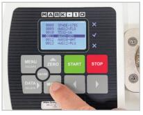
Save and recall multiple profiles, for quick and accurate switchover to different test methods.
