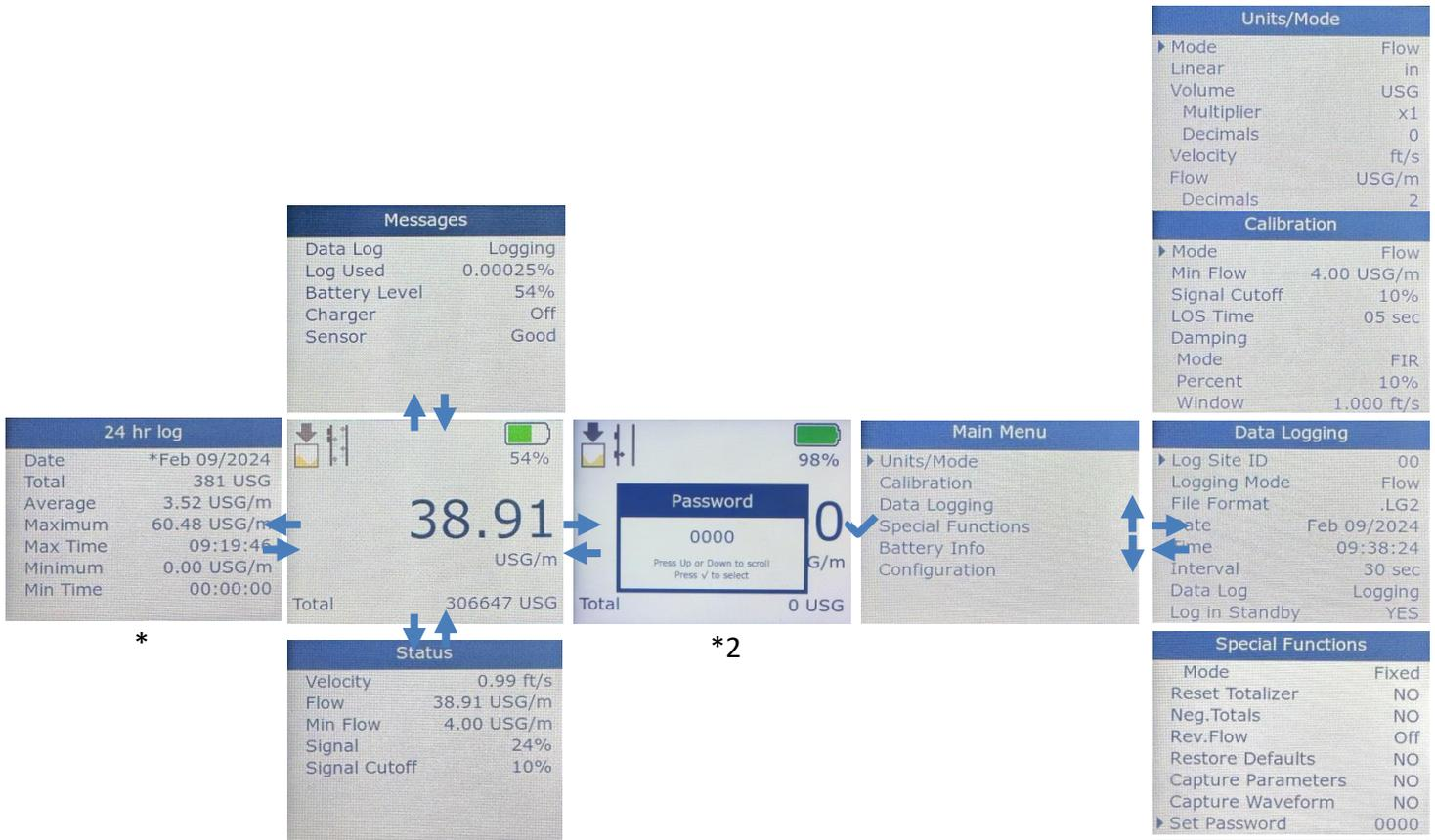
1 – Inserting a USB drive while on this page will download the 24 hr log data to the USB in .csv format
