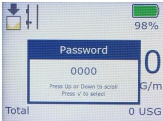
The password (a number from 0000 to 9999) prevents unauthorized access to the Main Menu for programming.
