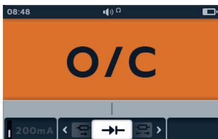
**NOTE :** The user is responsible for connecting test probes across the diode under test. There is no information displayed in the secondary field at this point. The only information to display is the diode drop voltage if the instrument senses a voltage across the device. If no current flows the main display will show "O/C".
