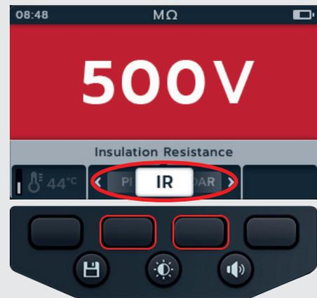
3. If required, press soft key 4 to toggle between temperature compensation on and off.
