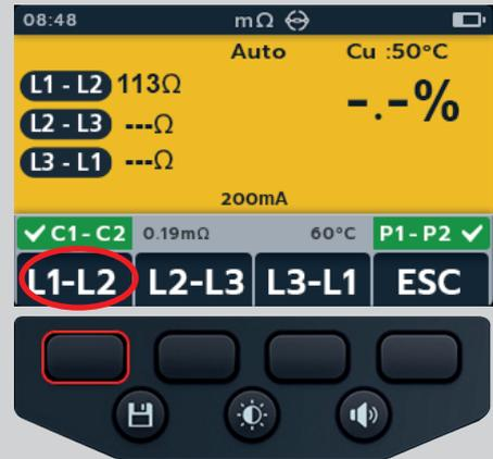
11. Press soft key 2 to assign reading to a phase (or press test before assigning to retest)
