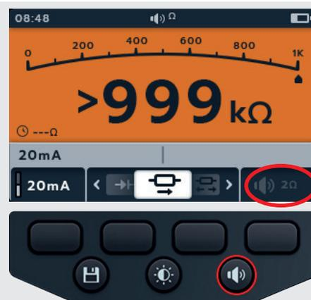
3. To adjust the continuity buzzer threshold press soft key 4.
