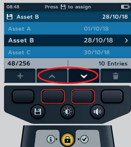
6. Press soft keys 2 and 3 to scroll up and down through the list.
