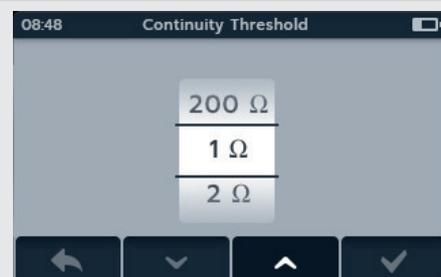
6. Press soft keys 2 and 3 to move the carousel left or right through sub-modes to uni-direction
