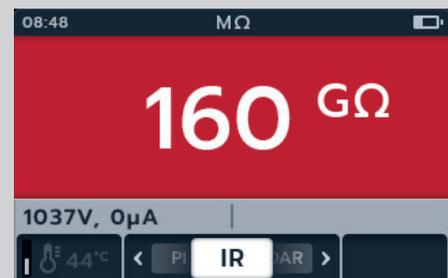
9. To save the test result press the SAVE button. A message will inform you the data was saved and which asset ID it was saved to.
