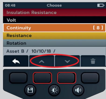
9. Press soft keys 2 and 3 to scroll up and down through the individual test list.
