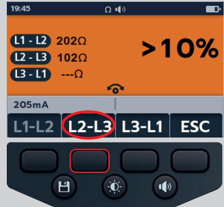
12. Press soft key 3 to assign reading to a phase
