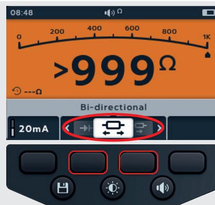
3. The test current can be toggled between 200 mA and 20 mA pressing soft key 1.
