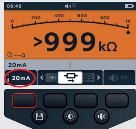
8. NULL the test leads by touching the two test probe ends. Press the TEST button until the NULL (symbol) appears on the screen. The ohmic value on the primary screen will read 0 Ω.
