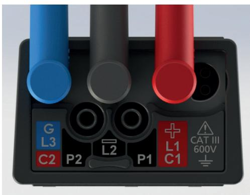
The guard lead (G) is optional. When used, it should be connected to the guard conductor, screen, steel wire armoured conductor, or "user added" conductive wire or wrapper, such as foil.
