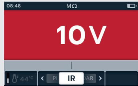
3. Press soft keys 2 and 3 to move the carousel left or right through sub-modes. IR is default, scroll through to 3P, PI, T(s) DAR.
