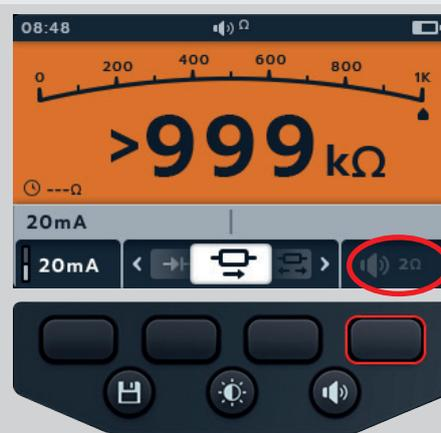
4. A new screen will open where the threshold can be adjusted pressing soft keys 2 and 3.
