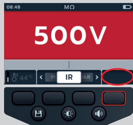
4. If required, Turn the buzzer OFF, ON-loud or ON-visual only as required by pressing buzzer button. Refer to 4.4 IR Buzzer settings on page 23
