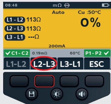
14. Press soft key 3 to assign reading to a phase
