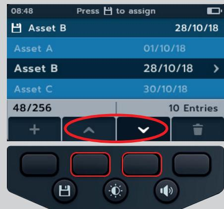
3. Press the SAVE button to assign the next measurements to this asset.
