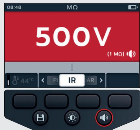
5. Start the test by pressing and holding down the TEST button. The buzzer will sound on test initiation.
