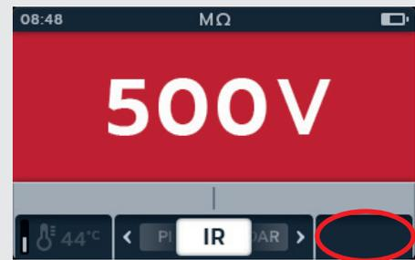
If a temperature measurement hasn't been made, the right of the secondary field will show -- °C.
