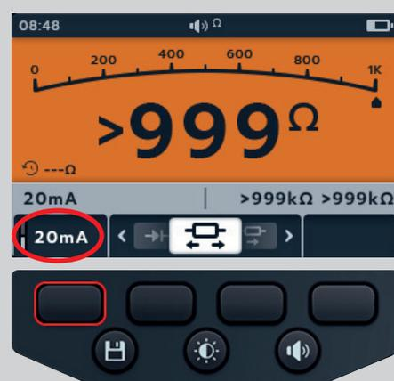
4. NULL the test leads by touching the two test probe ends. Press the TEST button until the NULL (symbol) appears on the screen. The ohmic value on the primary screen will read 0 Ω.
