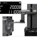
**Measurements**Simultaneous display of diameter and centerline
