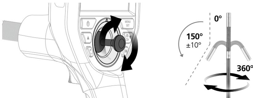
The factory setting for the maximum angular position of the 3D camera head is 150° in new condition, with a tolerance of  $\pm 10^\circ$ . To achieve this, the camera probe must be totally straight, meaning without any unnecessary curves or bends. The maximum angular position may be reduced by normal mechanical wear over the lifetime of the product.
