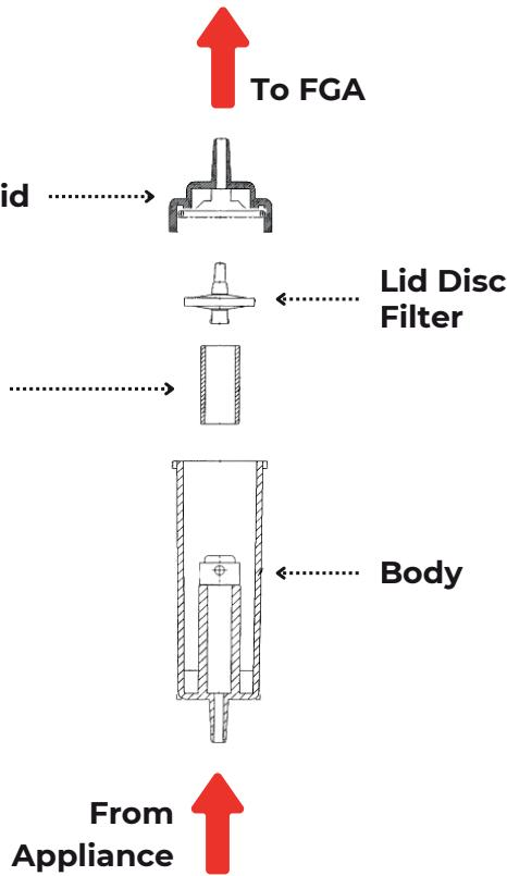
Please ensure the filters inside the Water Trap are clean, dry and assembled correctly.
