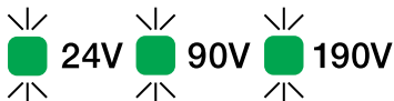
Figure 5.4 If the device is faulty, all the range indicators will flash simultaneously.
