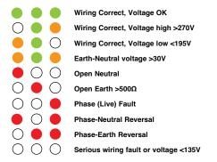
In the event of a fault being indicated, investigation should only be carried out by a suitably qualified electrician.
