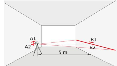
Then place the instrument at the same elevation as close as possible to wall A and again mark the horizontal laser line or the laser point on wall A (A2). Rotate the instrument by 180° again and mark the laser on wall B (B2). Measure the distances of the marked points A1-A2 and B1-B2. Calculate the difference of the two measurements.
