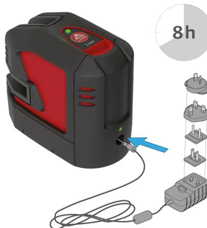
Charge the Li-Ion battery before using it for the first time. While charging, the instrument may heat up. This is normal and should not affect the instrument's lifespan or performance. At the recommended storage temperature of  $-20^{\circ}\text{C}$  to  $+30^{\circ}\text{C}$  ( $-4^{\circ}\text{F}$  to  $+86^{\circ}\text{F}$ ), batteries containing a 50% to 100% charge can be stored up to 1 year. After this storage period the batteries must be recharged.
