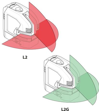
The instrument produces visible laser beams, which are emitted from the instrument. It is a Class 2 laser product in accordance with:
