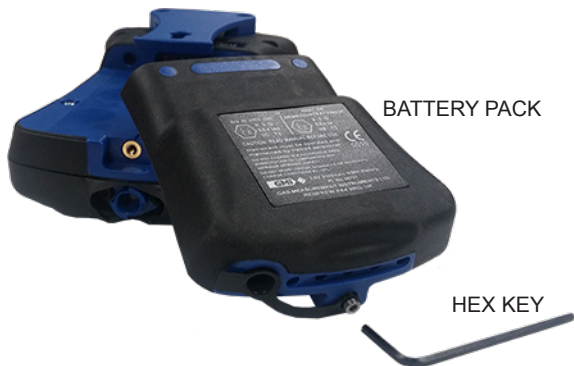
Fig. 4.11 Battery Pack Removed
