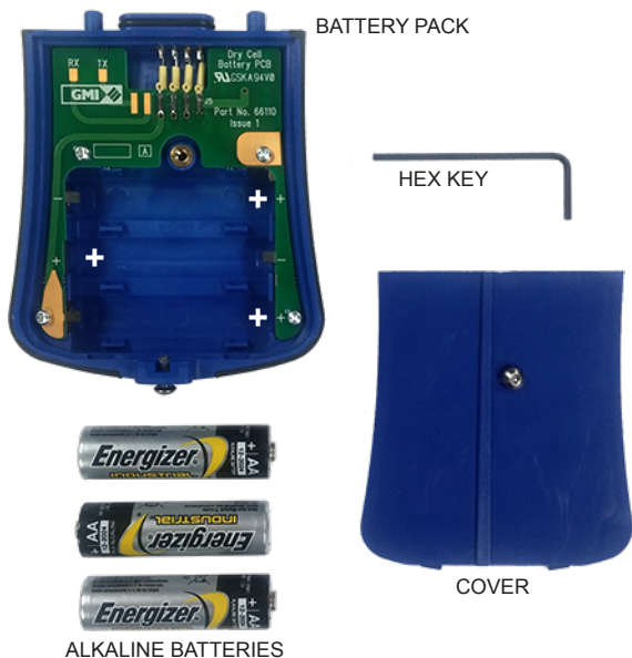
Fig. 4.13 Alkaline Batteries Removed
