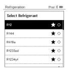
9.2 Setting the refrigerant: Press [▲] or [▼] to select the refrigerant and press [Menu/Enter] to confirm.
