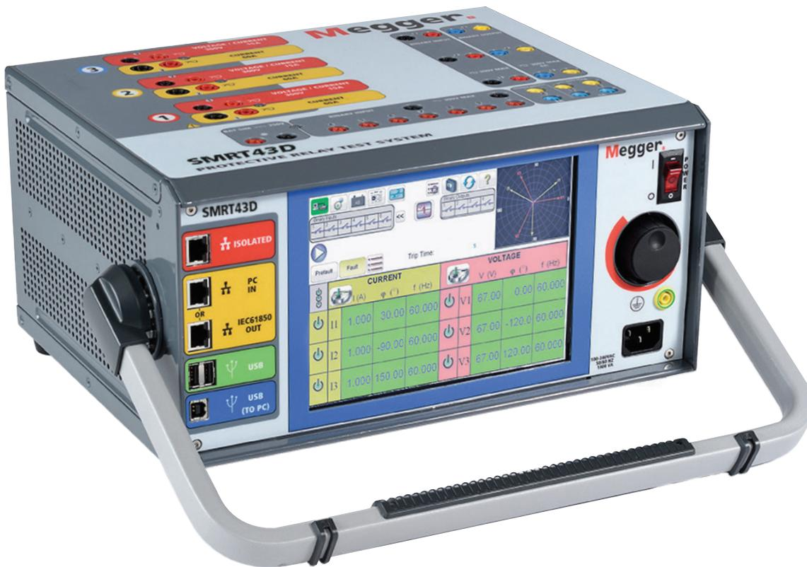
The "D" in SMRT36D and SMRT410D indicates these units include an integrated Smart Touch View Interface (STVI) providing stand-alone testing capabilities (no PC required)
