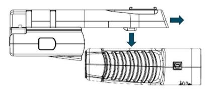
Figure 7-2. Attach the extension module
