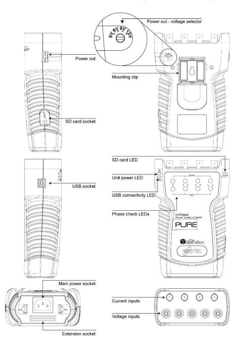
Figure 2-1. The analyzer connection & plugs
