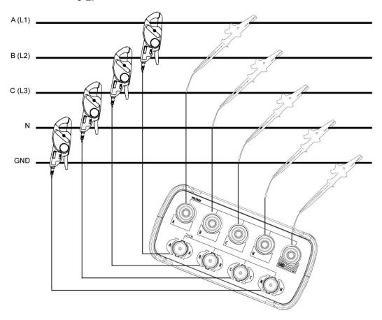
Figure 3-2. Connection of analyzer to 2-phase system
