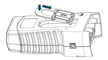
Figure 4-3. Fasten the mounting clip.
