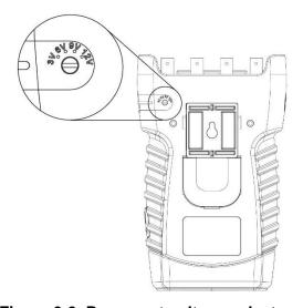
Figure 3-3. Power out voltage selector
