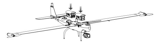
• Align the battery to the battery interface on the fuselage and install it.
