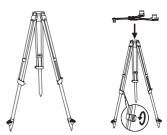
Install the base station body to the tray and tighten the lock on the tray nut. Ensure that the base station is level and stable.
