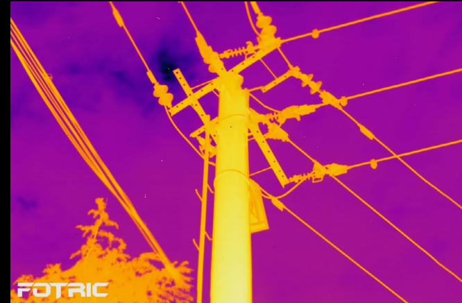
1280*1024 IR resolution (25° lens at 30m distance)
