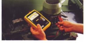
Checking the insulation of the windings of an electric motor
