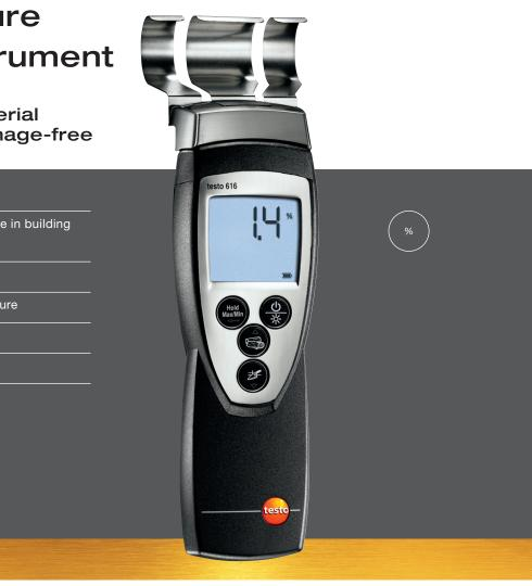
The test 616 allows fast and damage-free examination of material moisture curves in building materials and woods. It also facilitates your work in observing the drying process of floors walls and surfaces.
