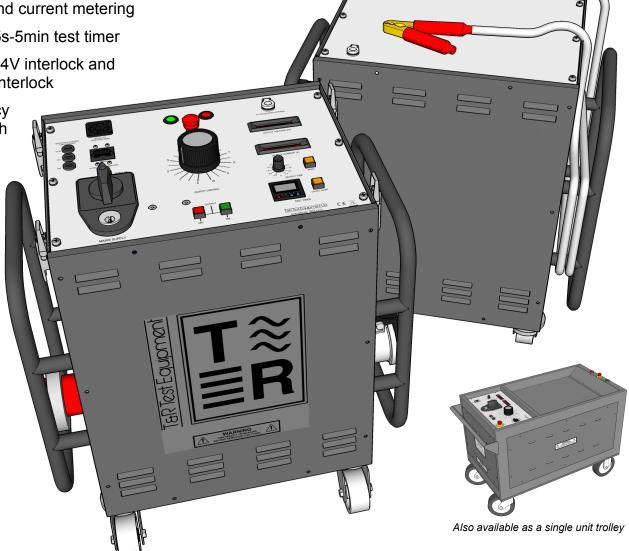
The HV trolley2 series of units are high power AC flash test sets with a 20kVA output capability. The maximum output voltage can be customised to be any voltage up to 15kV. The unit is housed in a rugged aluminium enclosure with a cover to protect the control panel. It is mounted on wheels to allow easy movement within a production environment.
