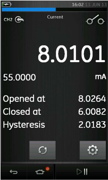
Figure 2-8 Switch Test Example
