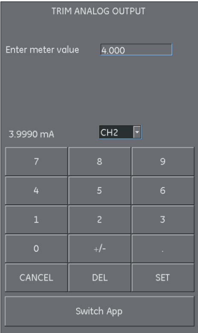
Figure 6-11 Enter Calibration Point
