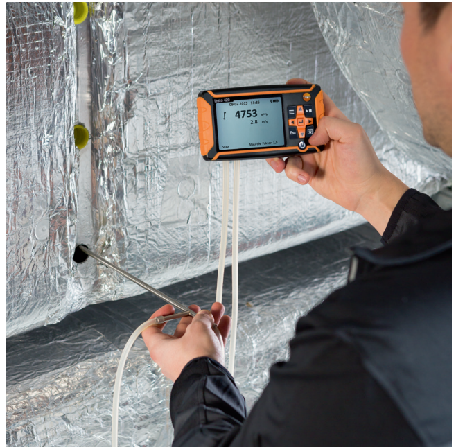
Removable instrument allows Pitot tube measurements in ducts (Pitot tube optional)
