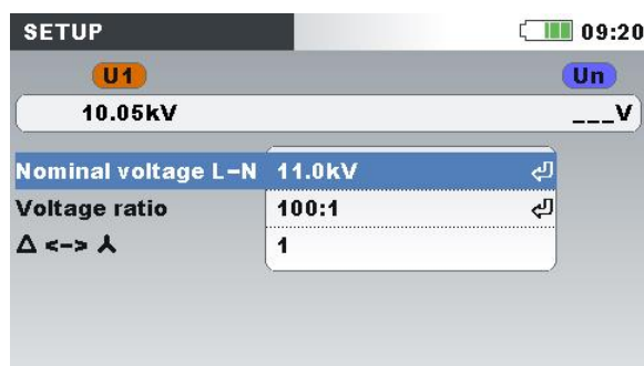
Figure 4.13: Voltage ratio for 11 kV / 110 kV transformer example
