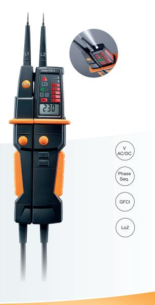
The testo 750 voltage testers are the first instruments to include an all-around viewable LED voltage indication. All three models include low input impedance, phase sequence, continuity test, and meet CAT III 1000 V CAT IV 600 V safety standards.
