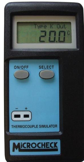
**INSTRUMENT OPERATION** - To turn the instrument on or off press the ON/OFF button. All display segments will be tested. The unit's resolution is 0.1 °C.
