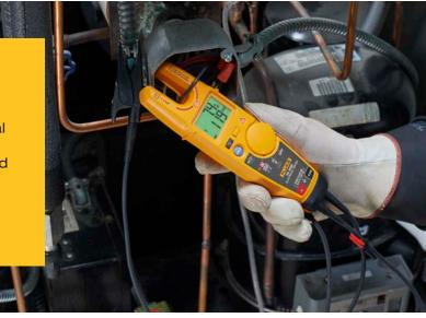
Thanks to the new FieldSense technology, the T6 makes work safer as you can measure voltage up to 1000 V ac through its open fork. Having the capability to measure voltage and current at the same time, together with eliminating the need to open covers or remove wire nuts, allows you to be faster and more efficient when taking measurements. In addition, the open fork is the widest available in the industry and can measure wires up to AWG 4/0 (120 mm<sup>2</sup>) carrying as much as 200 A.
