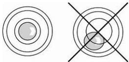
⇒ Level balance with foot screws until the air bubble of the water balance is in the prescribed circle.
