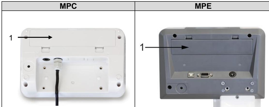
Open the battery compartment cover (1) at the base of the display unit and insert the rechargeable battery. Charge the battery for at least 12 hours before initial use.
