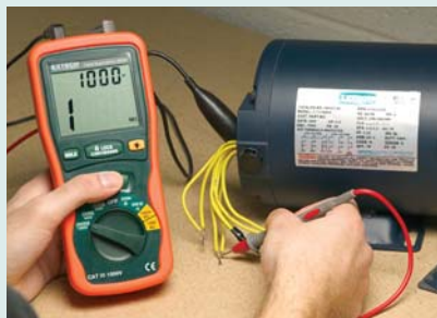
Measures the insulation resistance of motors
