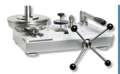
The deadweight tester (DWT) is a very robust and flexible pressure measurement standard. This guide is intended to simplify the process of selecting the right deadweight tester for your application. The following considerations will help you get started:
