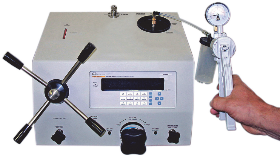
Figure 3: Evacuating the E-DWT-H with fill kit
