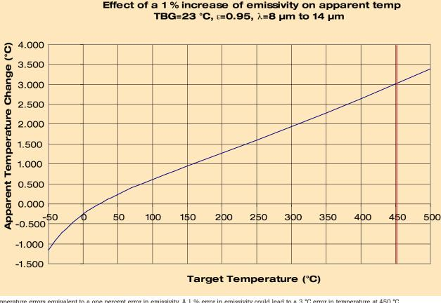
Temperature errors equivalent to a one percent error in emissivity. A 1 % error in emissivity could lead to a 3 °C error in temperature at 450 °C.
