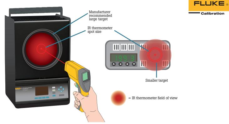
Peripheral vision in infrared thermometers makes large targets necessary for many calibrations.
