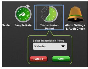
**Hint/Tip:** Hint/Tip: For a food service application a 1 hour transmission rate is fine.
