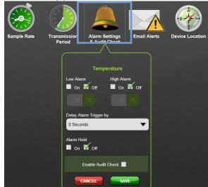
**Note**: When the Audit Check is selected it enables the user to identify when they physically visit the logger by holding down the button on the front of the device.
