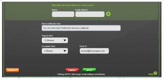
12 As changes are made to the settings of a data logger, they show in red on the 'Change Device Settings' screen. Once required changes have been made, click 'Apply' to action. The settings will transmit from the Cloud to the data logger at the next transmission period.
