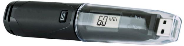
This standalone data logger measures and stores over 16,000 temperature and humidity readings from -35 to +80°C (-31 to +176°F) and 0 to 100%RH range at a resolution of 0.5°C (1°F) and 0.5%RH.
