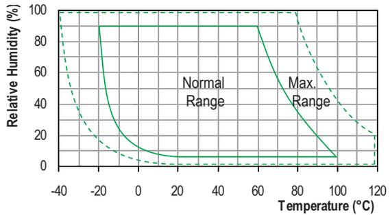
Long term exposure to humidity levels outside of the 'normal' range may temporarily offset RH measurements ( $\pm 3\%RH$  after 60 hours). Once returned to less extreme conditions the device will slowly return towards calibration state.
