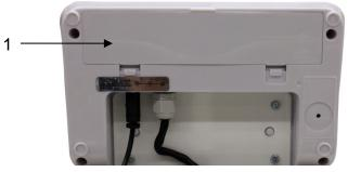
Open battery compartment cover (1) at the base of the display unit and insert battery. Charge the battery for at least 12 hours before initial use.
