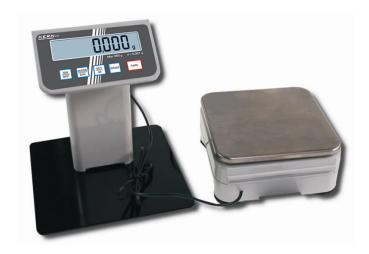
The balance must be installed in a way that the weighing plate is exactly in horizontal position.
