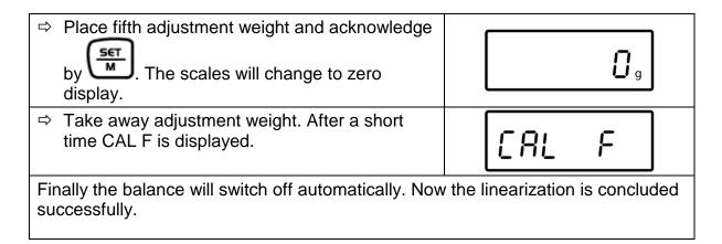
In case of an adjustment error or incorrect adjusting weight the display will show an error message; repeat linearization process.
