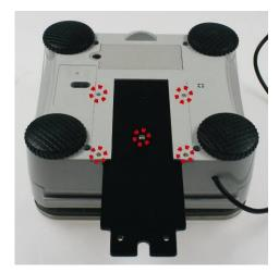
For disassembly remove the assembly sheet by loosening the marked screws. After that the display unit can be placed freely.
