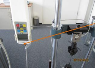
The plug of the external force gauge measuring cell has to be plugged into the socket of the FH force gauge.
