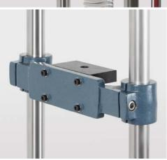
The external force measuring cell has to be mounted at the fitting bracket AFM 41 with an M12x40 screw (at TVM 5KN and 10KN) and with a M12x80 screw (at TVM20KN and TVM 30KN), included in delivery.
