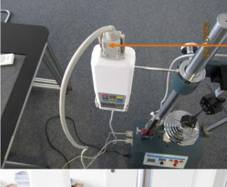
View from above FH with FH-A01 cable. A plug has to be inserted into the socket of the FH, the other one into the equipment port of TVM-N
