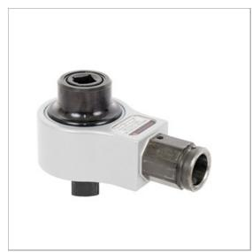
The HandTorque<sup>®</sup> HT3-1000 has been designed for use where it is necessary to provide higher torques than would otherwise be possible due to limitations of space or operator strength. Input to the multiplier is via a ratchet torque wrench set to one fifth of the desired output torque. **Part number**: 180260
