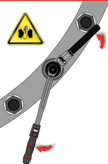
Before use, ensure the tool, socket and reaction are well maintained and not damaged in any way. Also ensure the retention pin is always fitted to the tool securing the appropriate reaction in place.
